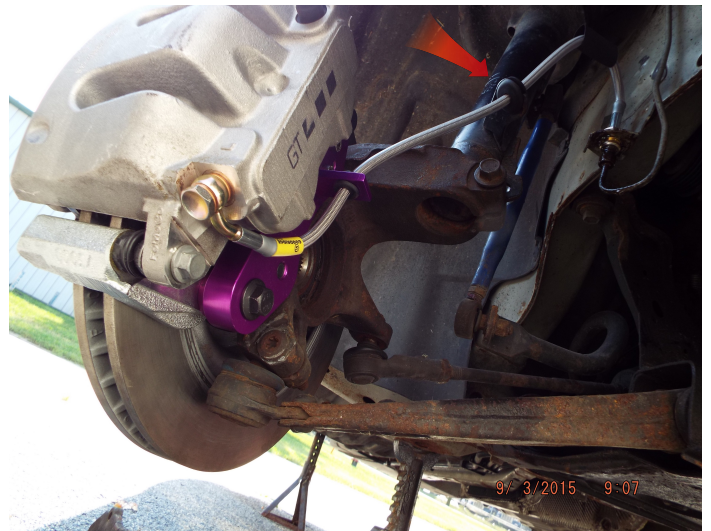
Illustration 12: Please CHECK your hose end configuration and make sure brake hose is correct for your installation. Slide large grommet into strut bracket
