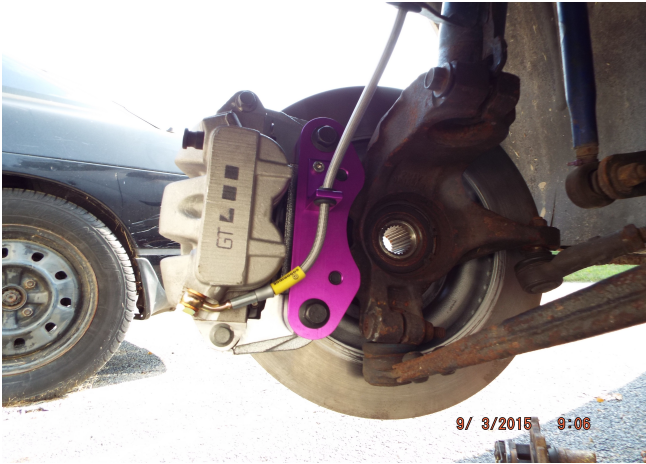
Illustration 10: Hose bracket attached to caliper conversion bracket.
