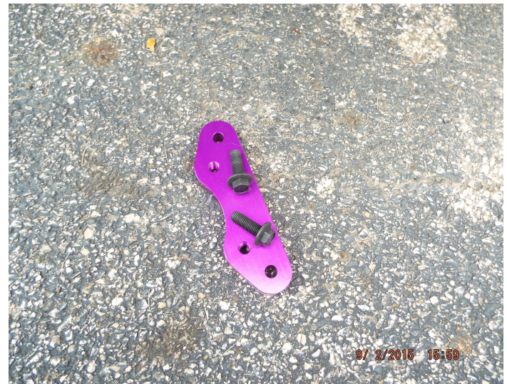
Illustration 2: Caliper conversion bracket and two M12 x 35 flange head bolts.
