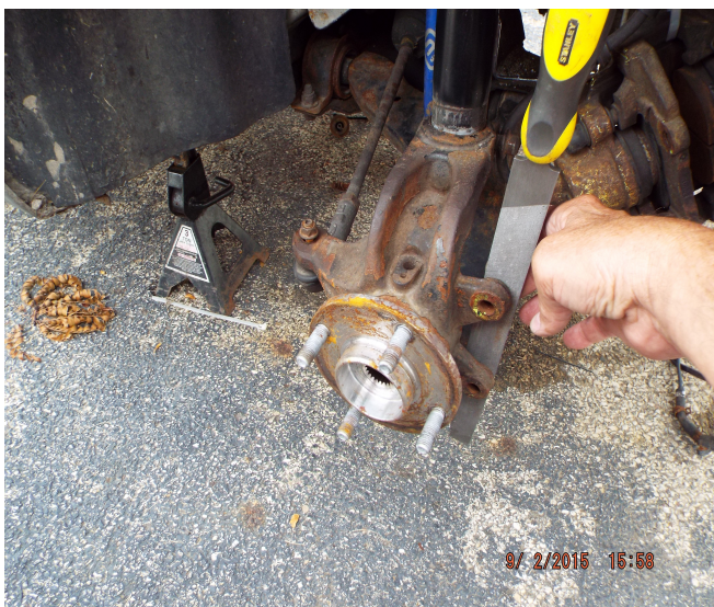
Illustration 1: Remove rust and debris from back of caliper mounting ears
