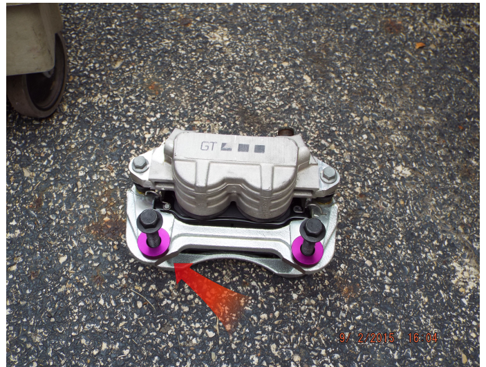
Illustration 6: Notice clearance has been ground on either side of caliper bracket near bolt holes.
