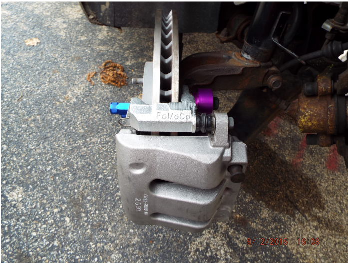
Illustration 8: Caliper TRIAL assembled to conversion bracket.
