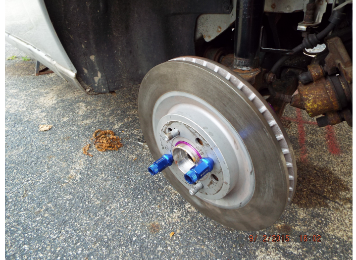
Illustration 5: Temporarily tighten rotor to hub.
