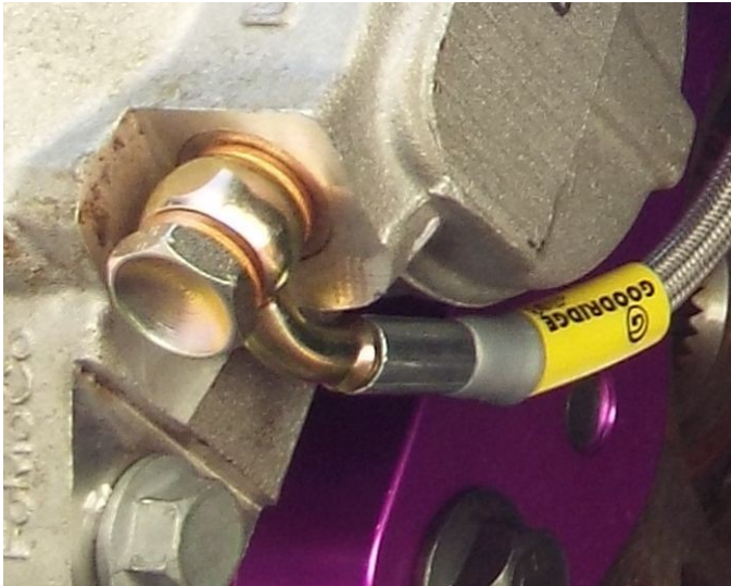
Illustration 11: Copper Washers on either side of Banjo fitting. Tighten to 25 ft/lbs.
