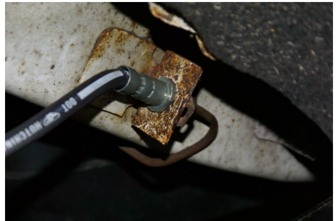
Fig. 15 Hose the chassis, clip installed
