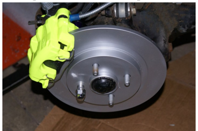
Fig. 10 Caliper w/ anti rattle clips
