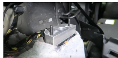
Fig. 6 Spacer Block in place
