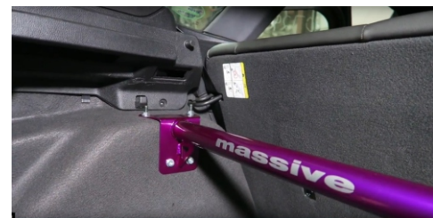
Fig. 9 Side Bolts Installed
