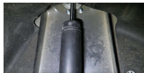
Fig. 10 Nuts installed from wheel well
