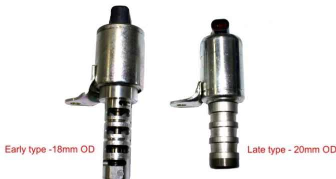
Fig. 6 VCT Solenoid Comparison
