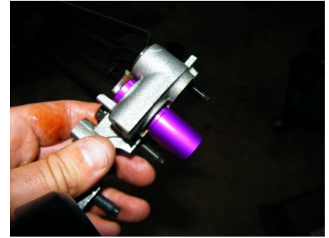
Fig. 4 Passage slug pressed in
