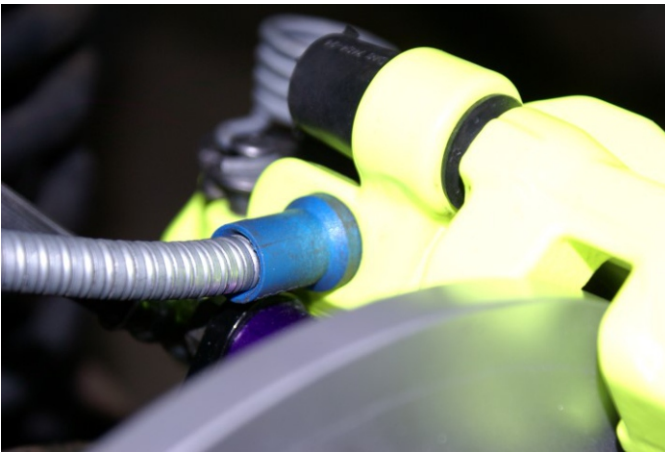
Fig. 13 Cable pushed into caliper (recommended). Torque to 85 Ft lbs).
