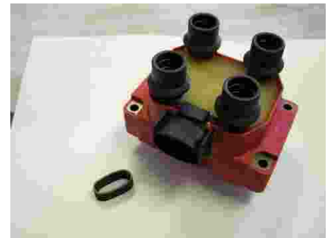
Fig.2 Gasket Ring Removed
