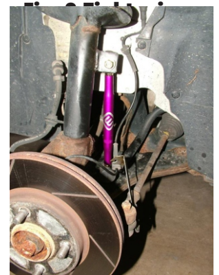
Fig. 3 New link installed
