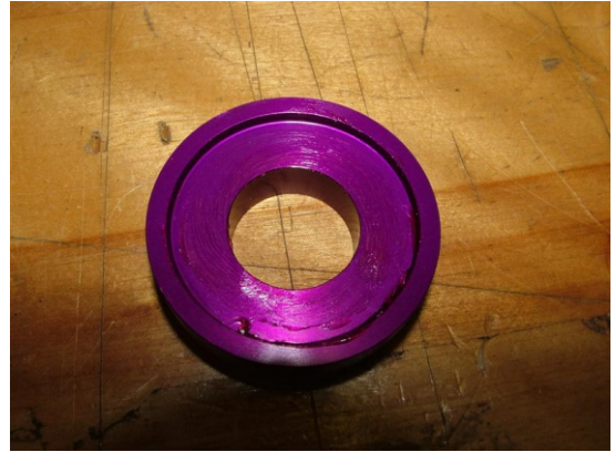
Fig. 1 Apply sealant inside
