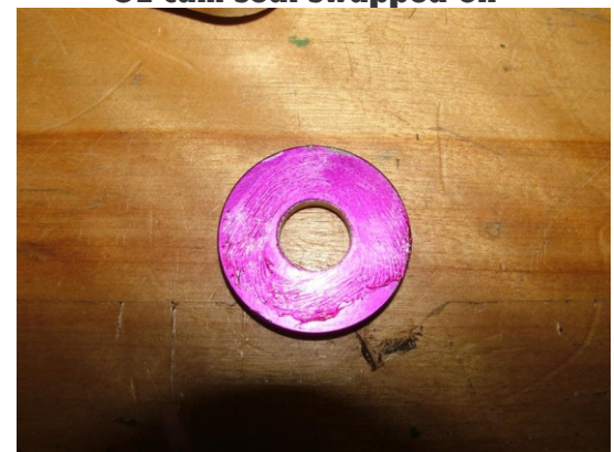
Fig. 3 Apply sealant inside washer
