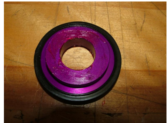
Fig. 2 Apply sealant outside, OE cam seal swapped on
