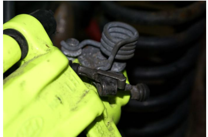
Fig. 14 Cable clipped to lever
