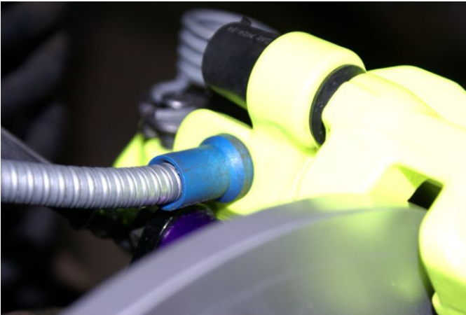
Fig. 13 Cable pushed into caliper
