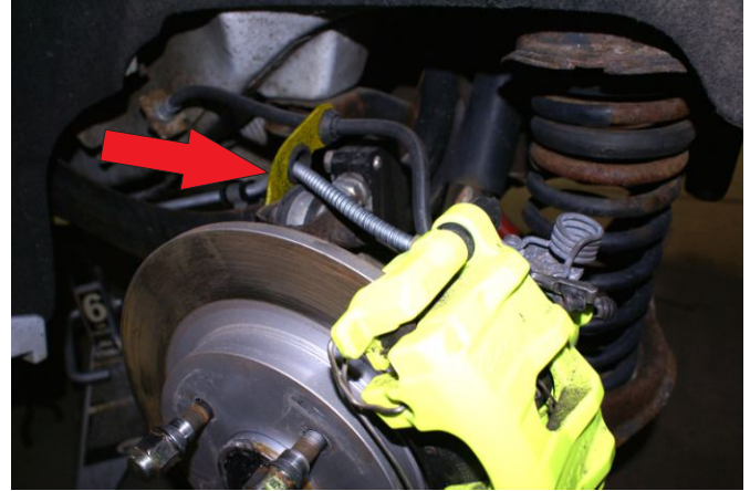
Fig. 12 Cable/ hose bracket
