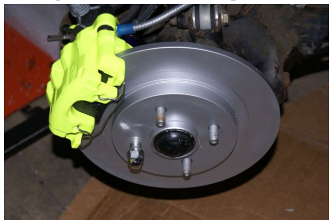
Fig. 10 Caliper w/ anti rattle clips
